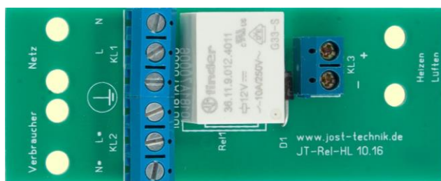
Illustration 2: Connecting Module JT-Rel HL to PHB
