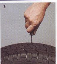
Thoroughly ream out hole with rasp tool
