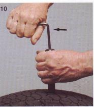
Then turn counter-clockwise until inner rod returns to bottom of Plugger
