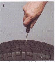
Use probe tool to inspect damage
