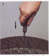
Insert probe and nozzle into the hole then unscrew probe from nozzle
