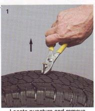
Locate puncture and remove damaging item
