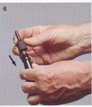
Slide nozzle over probe tool and screw down
