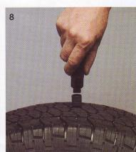
Screw loaded Plugger onto nozzle in tire
