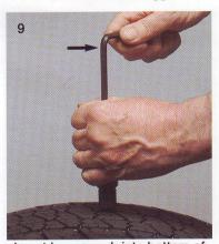
Insert hex wrench into bottom of Plugger and turn clockwise until it stops
