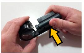
Push the lamp into the rectangular holder until et "snaps" into position, as shown to the left.
