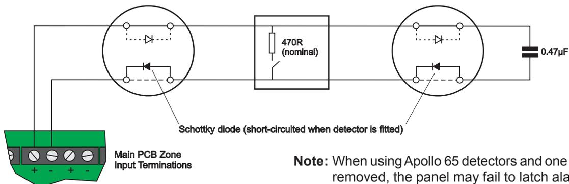
**Note:** When using Apollo 65 detectors and one has been removed, the panel may fail to latch alarms from
