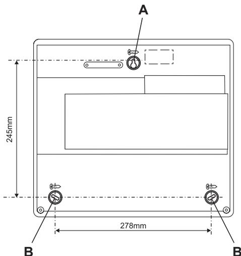
Overall Dimensions of panel in millimetres:
