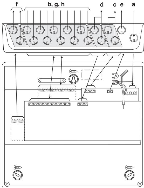
This section provides guidance on where to bring cables into the back box for ease of termination.
