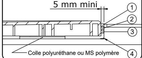
**FR-MISE EN PLACE DES PLOTS DE COLLE POLYURETHANE OU MS POLYMERE**
