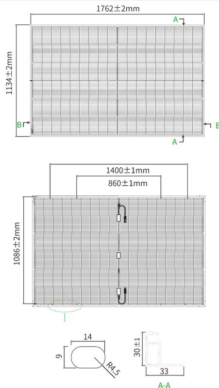
Noted: For specific dimensions and tolerance ranges, please refer to the corresponding detailed module drawings.
