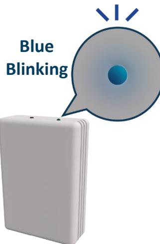
**Figure 2.7** WPS mode LED feedback.
