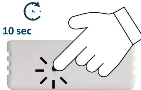
**Figure 2.4** Reset Wi-Fi procedure.
