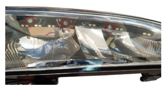
The emitter is fastened through the backside of the lamp, using the included screws.
