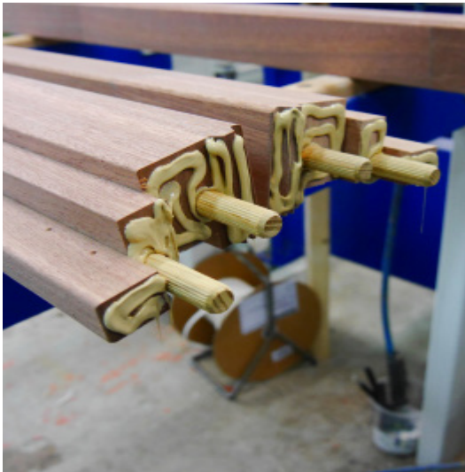
Figure 2: Applying adhesive in lines
