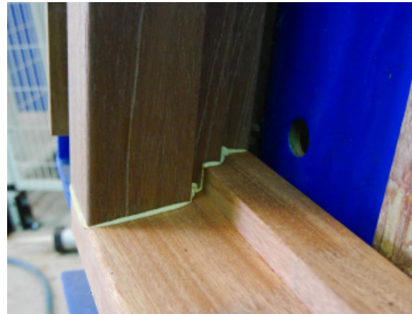
Figure 3: The adhesive is squeezed outwards.
