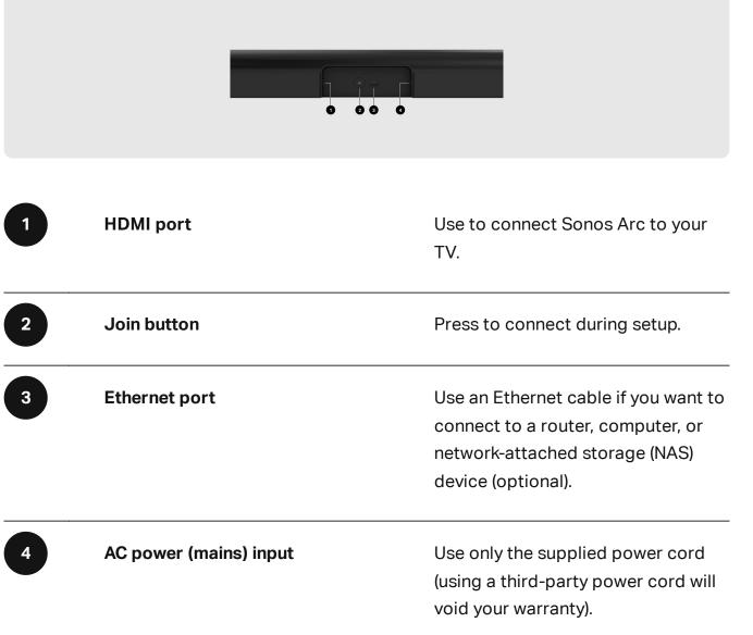
**Note**: Insert the power cord firmly until it is flush with the speaker.
