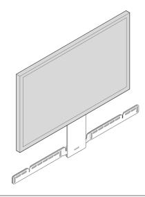
If your TV is wall-mounted, place the positioning guide against the wall, aligning the top edge with the bottom of your TV. There should be 5.5" (140mm) between the top of the wall mount bracket and the TV.
