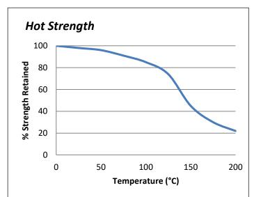
"Hot strength" shear strength tests performed on mild steel. Fully cured then conditioned to pull temperature for 30 minutes before testing. ES5501 can withstand higher temperatures for brief periods (such as for paint baking and wave soldering processes) providing the joint is not unduly stressed. The minimum temperature the cured adhesive can be exposed to is -40°C (-40°F) depending on the materials being bonded.
