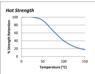
"Hot strength" shear strength tests performed on mild steel. Fully cured specimens conditioned to pull temperature for 30 minutes before testing at temperature.
