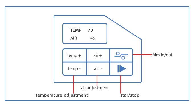
Different film type requires different air volume, speed and temperature. Please select the correct film type firstly.
