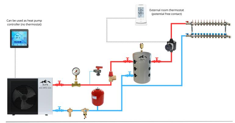
Installing multiple automatic air vents in the heating system is crucial for optimal performance and longevity. These vents efficiently eliminate trapped air, preventing uneven heating and potential damage. This straightforward enhancement significantly boosts system efficiency and comfort.
