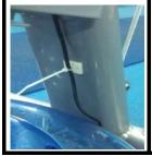
4. The excess lead can be stored under the Perspex cover.
