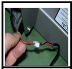
1. After confirming all parts are present. Stand the rower into the vertical position and attach the long lead at the front of the rower as shown.
