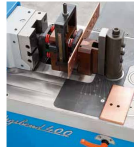
Punching unit for holes up to \varnothing 30 mm. Max thickness 12 mm.
