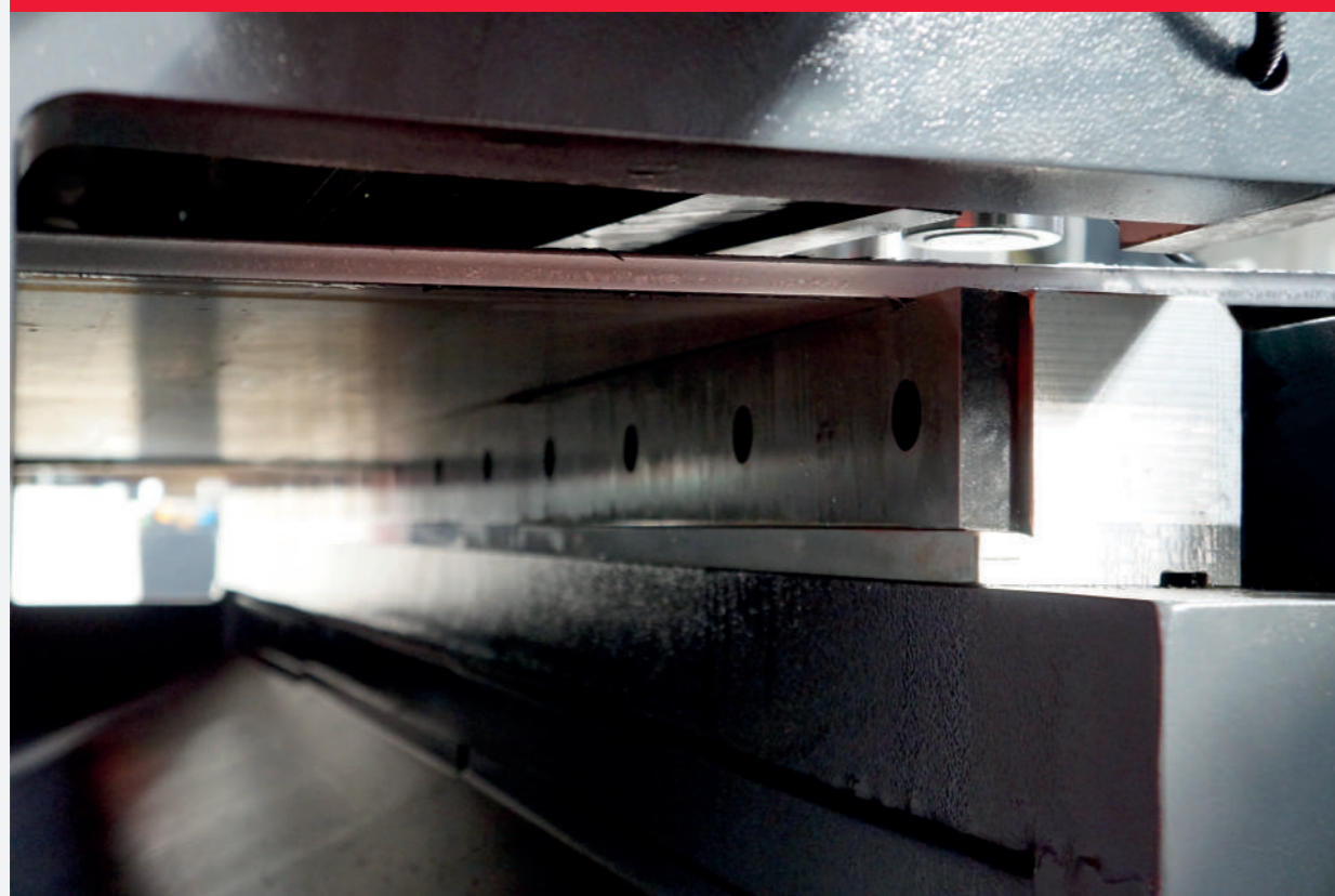
Excellent cutting quality from 6 mm up to 20 mm with powerful monoblock body
