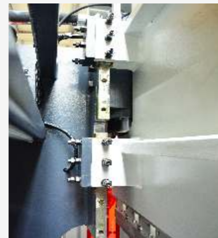
Stronger Beam Guiding System to stable the beam
