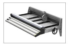
The infeed guide roller are angled to match the loop of the coil from a decoiler. This helps prevent creasing on soft materials like copper, aluminum and zinc.
