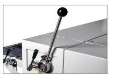
The EASY series has 3 manual straightening rollers to remove coil set and give customers flat material every time. The rollers are made of polished steel with a 70 mm diameter. The pressure of the straightening rolls is set by locking handles with reference scale.
