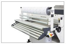
Optional: The film applicator can basically be mounted on any table. Using the deflection rollers and the fully rubberized feed rollers, the protective film is pressed on almost bubble and wrinkle-free. The decive type F-AG z2mo has an additional arm with tension spring for tensioning the film during the return movement. This design is only applicable for single decoiling systems. The film applicator is available in both 50" (1250 mm) and 59" (1500 mm).
