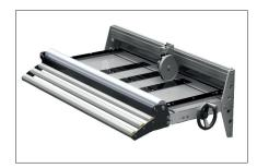
The infeed guide roller are angled to match the loop of the coil from a decoiler. This helps prevent creasing on soft materials like copper, aluminum and
