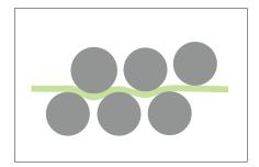
The STRAIGHT machine has 6 manual straightening rollers to remove coil set and give customers flat material every time.
