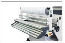
Optional: The film appicator can basically be mounted on any table. Using the deflection rollers and the fully rubberized feed rollers, the protective film is pressed on almost bubble and wrinkle-free. The device type F-AG z2mo has an additional arm with tension spring for tensioning the film during the return movement. This design is only applicable for single decoiling systems.
