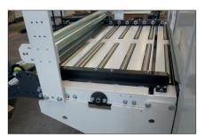
Optional: The coil guide is an important component for the function and accuracy of every system. The table has a fixed and a manually adjustable coil guide with ball bearings. The adjustment of the movable coil guide is done by a hand wheel. This specific table has rollers integrated in the table to ensure a smooth surface.
