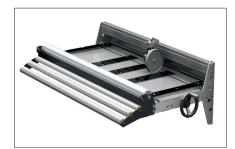
The infeed guide roller are angled to match the loop of the coil from a decoiler. This helps prevent creasing on soft materials like copper, aluminum and
