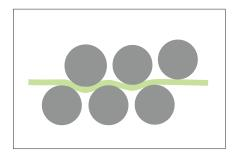
The POWER STRAIGHT PRO has 6 automated straightening rollers to remove coil set and give customers flat material every time.
