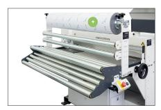
Optional: The film applicator can basically be mounted on any table. Using the deflection rollers and the fully rubberized feed rollers, the protective film is pressed on almost bubble and wrinkle-free. The device type F-AG z2mo has an additional arm with tension spring for tensioning the film during the return movement. This design is only applicable for single decoiling systems.
