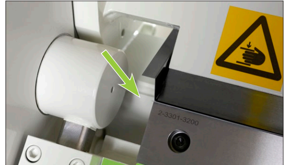
Large recesses in the clamping beam.
