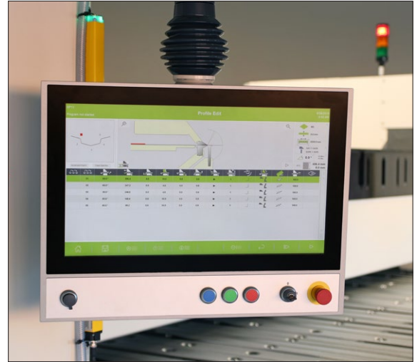
FORMA Z as standard equipped with ProLink W with 21.5" screen on a pendant arm.
