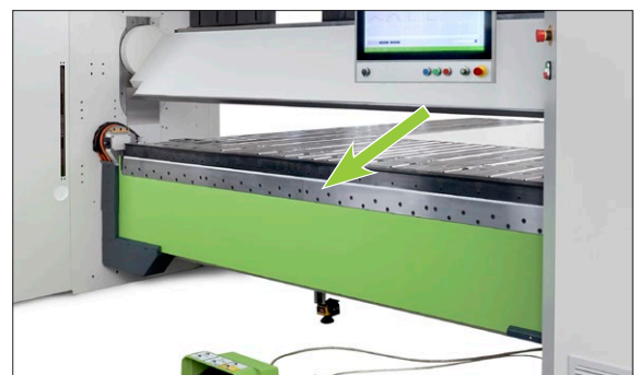
CNC controlled crowning.
