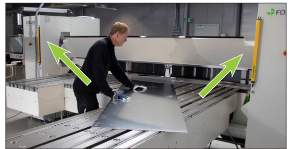
Light guard on gauging side.
