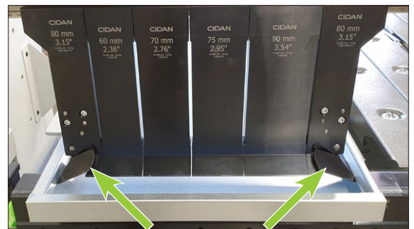
Collapsible corner tools for manufacturing of boxes and doors.
