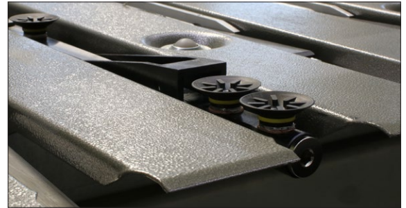
Vacuum grippers in the back gauge.
