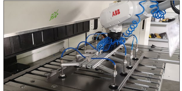
Folding machine served by a robot.
