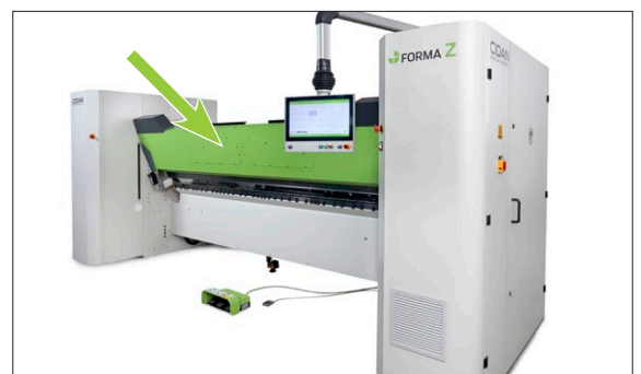
Sturdy folding beam in upper position.
