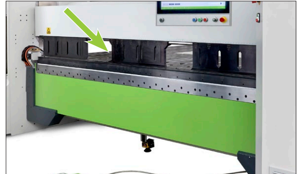
High divided box tooling 203 mm.
