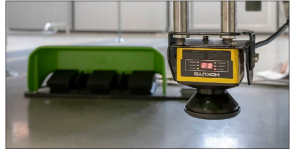
Laser scanner mounted in the folding side.
