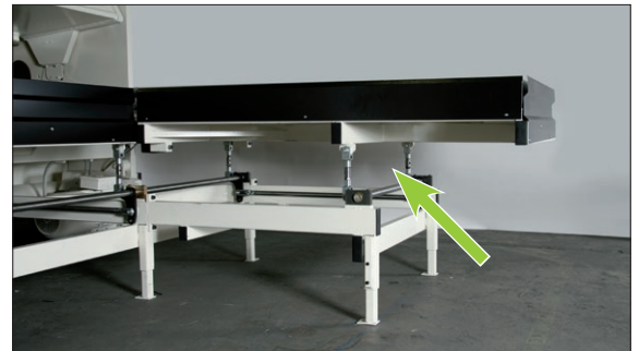
Height adjustable back gauge for Multifold.
