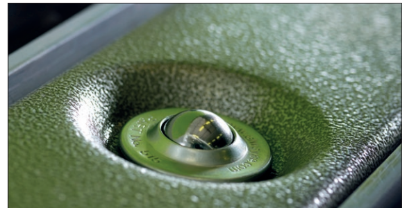
Steel ball transfers standard on AGS back gauge.
