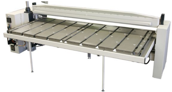
EGS back gauge 1020 mm, steel ball transfers are optional.
