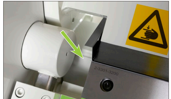
Large recesses in the clamping beam.
