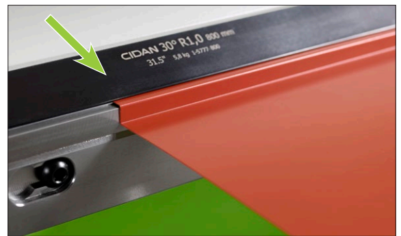
Straight rail 30° with radius 1 mm.
