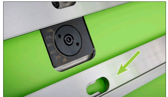
Quick changes thanks to the bayonet tooling system.
