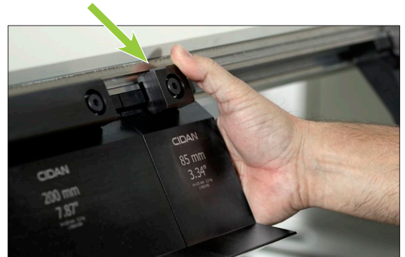
Box tools with fast locking, easy to move.
