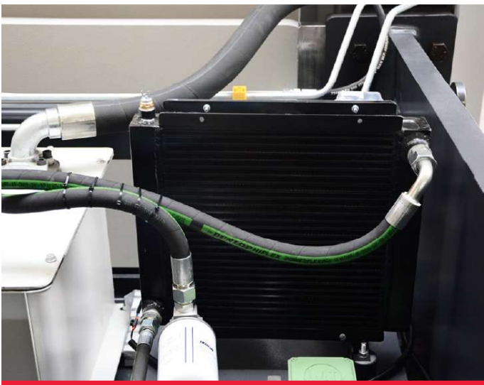
Hydraulic Oil Cooler System
