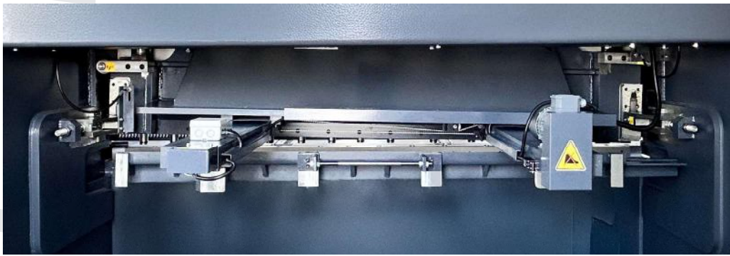
Motorized Back Gauge has \pm 0,1 mm Accuracy
