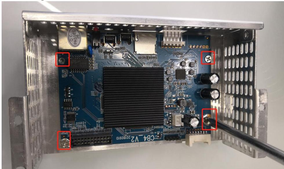
2) Insert the power control cable and the adapter board control cable into the corresponding slots on the control board, and then fix the bracket to the chassis with screws, as shown in the figure:
