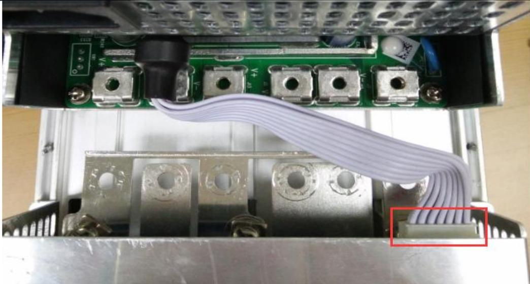
2) Then connect the 6 positive and negative terminals on the power supply to the copper row one by one, and then install 6 screws in turn. The screws should be tightened and the washers should be aligned parallel to the edge of the copper bar to avoid short circuiting the power supply or the power board, as shown below:
