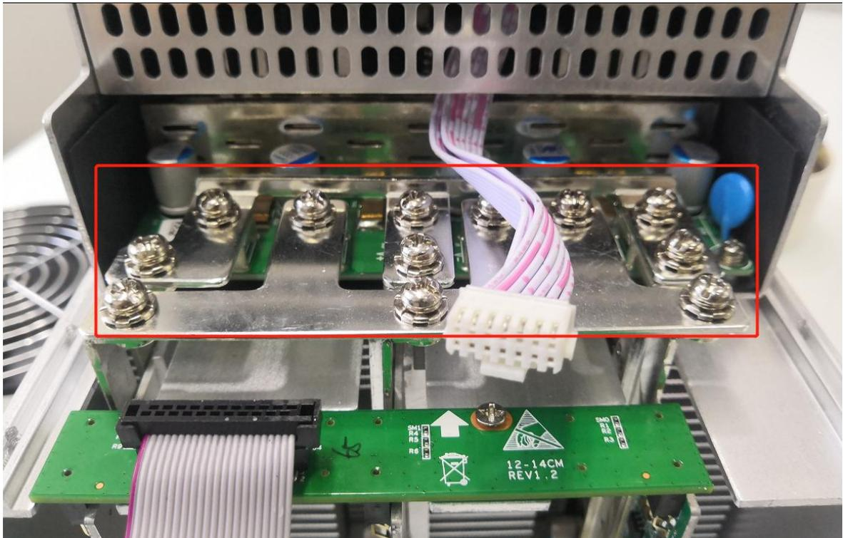
4) After the power bridge is installed, then install control board and the fans, finally the whole hash board installation is done.
