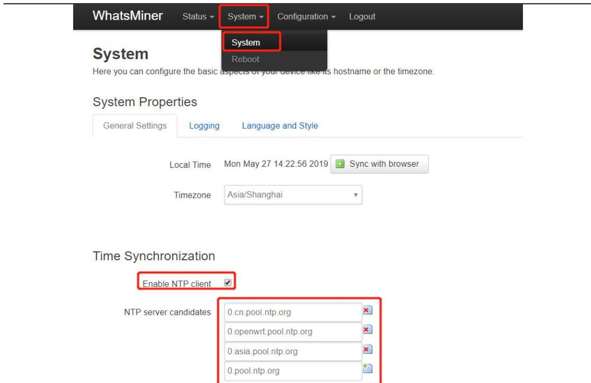
(2) In the miner configuration interface, add or modify the NTP server address. The miner has been configured with four NTP server addresses by default. You can modify or add the NTP server address to the local NTP server address according to the mine situation.
