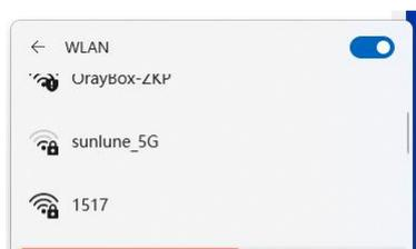
c) After connecting to the Jasminer machine' s Wi-Fi, open your web browser, enter the address "83.85.78.1" and click Enter and Login to the backend console
