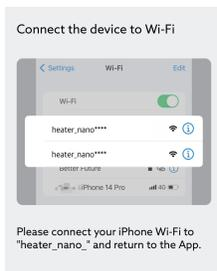
After clicking the plus sign in the upper right corner, follow the prompts to enter the mobile Wi-Fi settings and select the Wi-Fi named heater\_nano\_\*\*\*\* to connect. This process does not require entering a password. After successfully connecting, switch back to Avalon Remote App and click Next step.
