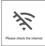
This symbol on the screen indicates that you need to check if the IP address is displayed correctly. If it is expected, then troubleshoot the current Wi-Fi failure. Please check the settings, such as carrier, mining pool configuration, or VPN.
