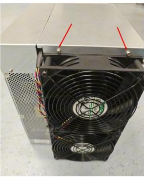
2. Remove the two upper covers and unplug a total of 9 cables on the control board, including the operation board arrangement cables, the fan cables, the control board power supply cables and the power supply voltage regulating cables, as shown in
