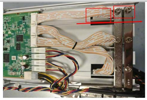
4. Remove the cables and screws, the rest of the hash board can be extracted, as shown in the figure:
