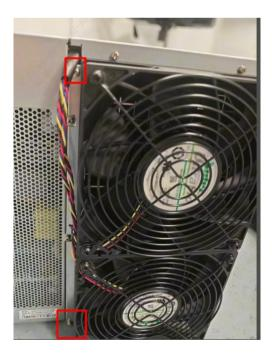
3. Pull out the cable of the hash board, unscrew two screws on the copper bar, and the hash board can be pulled out, as shown in the figure:
