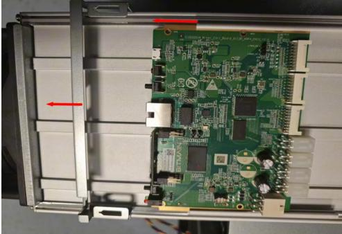
and push the control panel along the chute, as shown in the figure:
