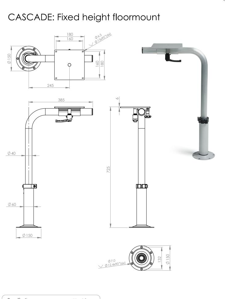
Specifications: Material and finish: Aluminum anodised Steel **powdercoated**
