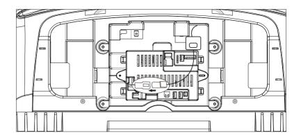
9. Install the two side panel plastic parts: first hook the upper steel pipe , then fix it with 4×12 flat head screws in the right position on the bottom of the go cart.
