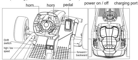
**Warning:** Please make sure the switch is in the disconnected mode, that is the driving mode, it is safe for the beginner.
