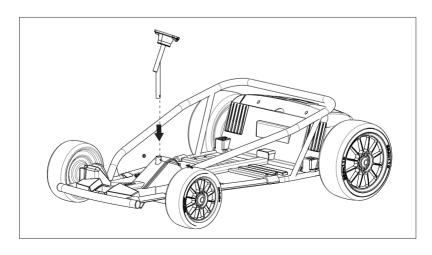
2). Insert the steering axle from the bottom to the car body and steering axle holder, until the top of the steering axle extends out the steering axle holder.
