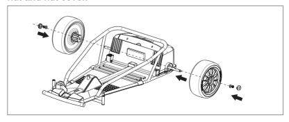
After the rear wheel is installed, turn over the body and tighten the screws that hold the rear axle.
