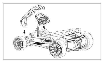
8.Remove the 2 screws and open the trunk lid, then connect the power wire's butt joint, cover the lid and fix it with the 2 screws.
