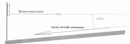
When the street is a slope or the radar is tilted, so the measurement vector is not paralell to the traffic vector, the sensed speed is less than the actual vehicle speed.
