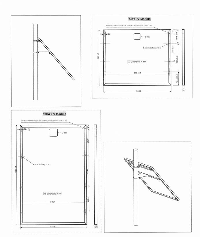
Note: The solar panel should be directed to South. If there is no possibility to do this and the solar panel is directed to North, you will loose at least 60-70 % power of solar panel.
