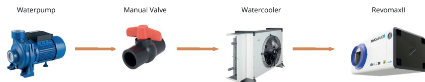
Manual valve install sequence
