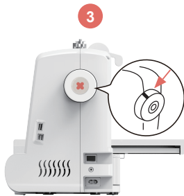
Reset the handwheel to ensure the needle in the highest point
