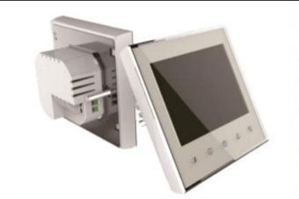
The connection must be carried out by a recognised installer in accordance with the NEN 1010 regulations. Before installing or disassembling the controller, always switch off the electricity in the control cabinet. The Quality Heating thermostats can be installed in a single flush-mounting box with a depth of 5CM according to standard DIN formats. Always check that the power has been switched off.
