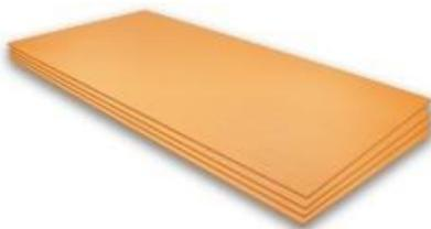
The ISO74 increases the efficiency and response time of the underfloor heating foil. These properties result in lower energy consumption. The ISO-74 can only be installed on a flat subfloor. Tape the corners with tape to prevent slipping. Leave approx. 30 mm space for the supply wires. Make sure that the floor is clean and that no sharp objects can get in contact with or fall on the heating foil during installation.
