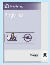
In monitoring mode, the brightly lit LCD screen displays patient name, battery life and wall-charging state.
