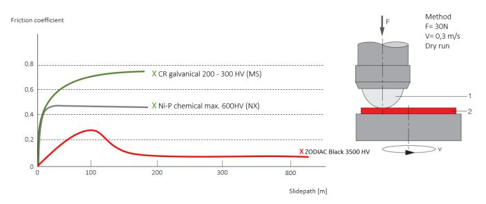
In this comparison test we see the sliding wear of different nozzle suppliers. The diamond specimen (fig.1) is pressed with a contact pressure of 30N with a speed of 0.3mm/s onto the coated specimen (fig.2).
