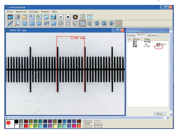
Enter the actual distance value, and the corresponding unit. The calibration is done. This calibration can be used to measur at this magnification.
