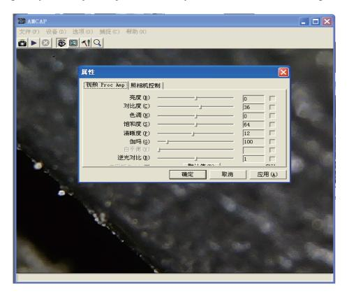
note: in the amcap software, the 'ZOOM' button can increase the magnification 5 times; and double click or long press 'SNAP' button can take photo. Set photo save path: seclet 'capture', 'set image path'.
