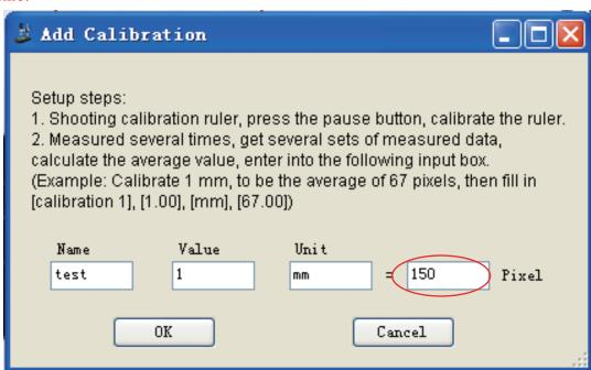
Calibration done, do not make any changes to the microscope, replace object with the calibration ruler and put it in the right position before the microscope. Click to take pictures. Double click on the image, then you can measure it. The software can measure various points, lines, shapes, length, angle, radian and other parameters. Measurement results can be exported by Word or Excel, mail.
