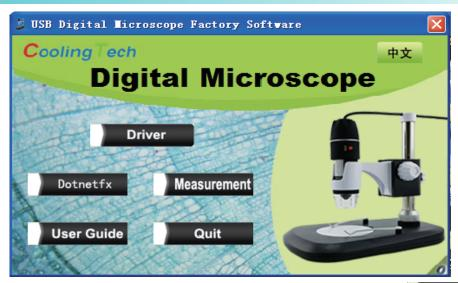
Please connect the product to your computer before installation.click measurement Measurement, or open CD,double click Measurement.exe,select 'next' —setting setup path,select 'next'—select 'close'.In the installation process,if system prompt need to install 'Net framework V2.0',then open the 'dotnetfx.exe' in CD, to install Net framework V2.0, then you can successfully install measurement software.
