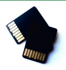
For recording at sample rates between 16kHz and 48kHz, a microSD card with a speed class of 10 or greater is required to make sure the cards keep up with the device.
