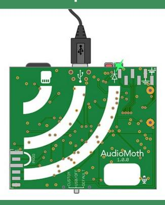
Set the switch on the side of your AudioMoth device to USB/OFF and attach it to your computer via USB.
