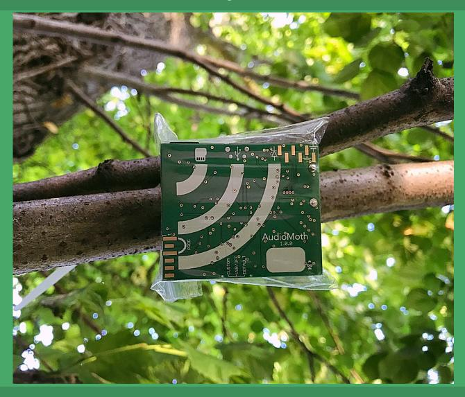
With the AudioMoth configured and the switch in the CUSTOM position the device can now be deployed in the field.
