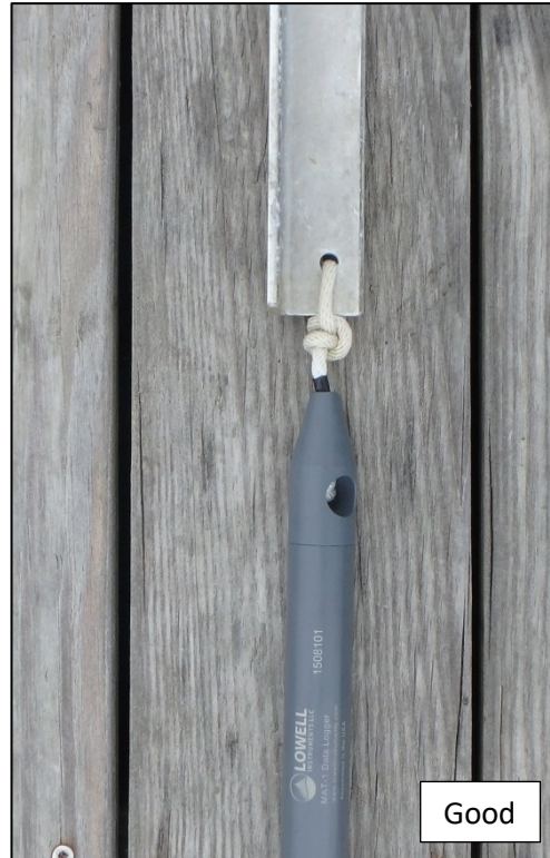
Figure 3A (top left): The recommended mounting method for an aluminum bracket is to drill through the bracket, deburr the hole and knot on the back side.
