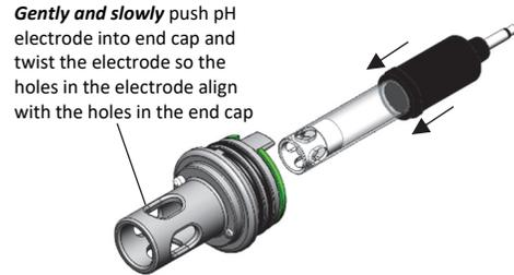
6. Continue to gently push the electrode into place until the clear plastic is fully seated in the end cap as shown.
