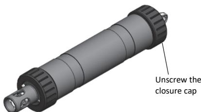
3. Pull the mounting end cap and attached battery holder straight out from the logger body without twisting. Insert a screwdriver through the mounting hole if you need additional leverage for removing the mounting end cap from the logger.
