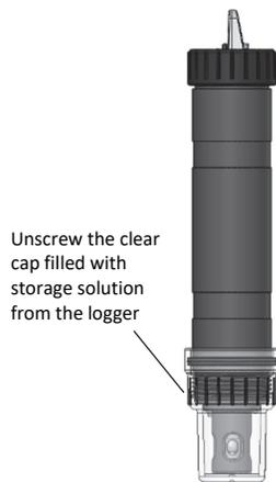
2. If you removed the clear storage cap, screw the closure cap onto the logger.
