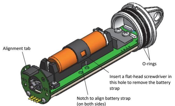
5. Remove the battery and install a new one, observing polarity.
