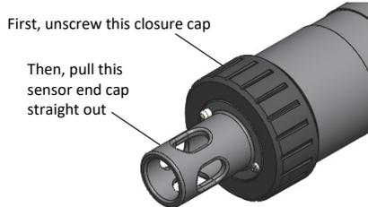
2. **Gently and slowly** remove the pH electrode from the sensor end cap. (**Note:** Removing the electrode too quickly could result in unseating the internal O-rings.)
