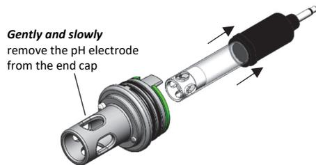
3. Use a foam swab dipped in water to clean the internal O-rings. Use the foam swab to spread a small dot of silicone-based grease along both the O-rings inside the sensor end cap. Do not use a cotton swab as the fibers on the swab can interfere with the operation of the electrode.
