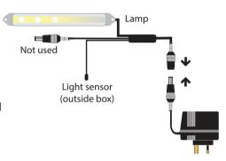
When using this camera kit you need to run a separte power supply for the lamp, unless you are powering the camera using a 12V power supply.
