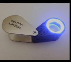
7. Switch LED on to confirm batteries are placed correctly
