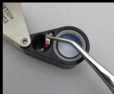
3. Carefully lift electrode and wiring from compartment (use paperclip/ tweezers)
