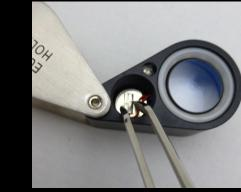
5. Place electrode on top of batteries
