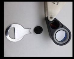
2. Unscrew lid with enclosed tool or coin to access battery compartment
