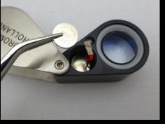
4. Stack batteries into compartment, make sure that positive charge (text) is facing upwards
