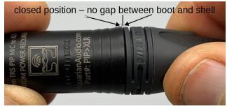
Tighten the chuck by turning the boot clockwise until snug. Hand tighten only. Note that there should be no gap between boot and plug when tight. Test by gently pulling on the hydrophone cable.
