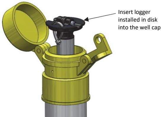
4. Close the well cap. Use the cable tie as a handle to pull out the logger and disk as needed.
