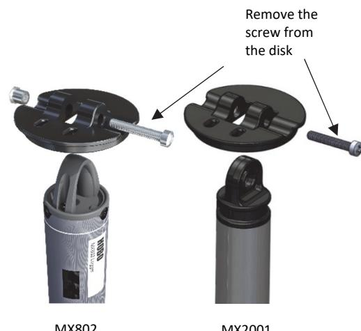
2. Insert the top end of the logger into the opening between the two raised holes on the disk. Slide the screw through all three holes and tighten it with a screwdriver. Attach the cable tie to the disk by feeding it through the two side holes as shown below.
