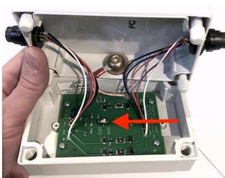
3. In the center of the circuit board, use the switch to select the appropriate Song Meter model:
