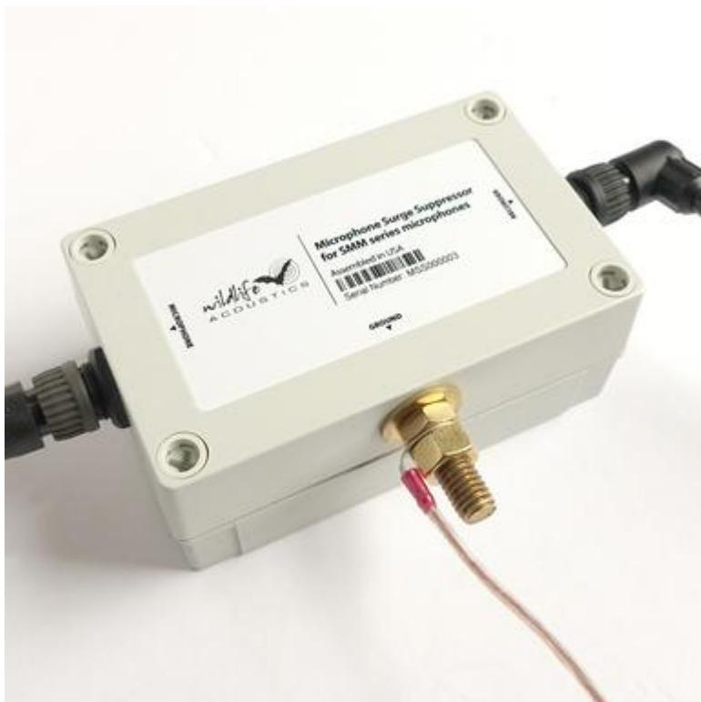
The Song Meter Surge Suppressor protects SM4, SM4BAT, SM3, and SM3BAT recorders from power surges due to electrostatic discharge or electrical storm activity that could travel down the microphone cable and damage the recorder.
