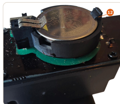
Figure E · The battery and its clip
