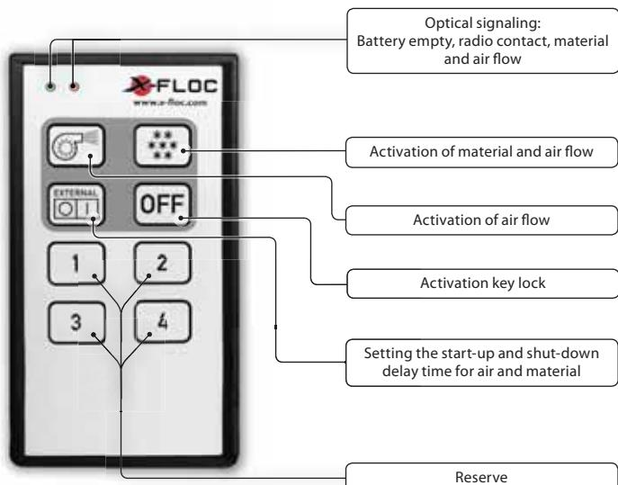
The machine type M99-DS-Pro and M99-DS-Pro 8K is supplied as standard with a specially developed radio remote control FFB2000-Pro. All important settings and functions can be comfortably controlled from the operator's workplace. The air power and the material flow volume can be adjusted in 19 levels during operation or in standstill.
