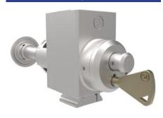
S40 IR Escape Release Adaptor module is used in conjunction with a releasing amGardS40 unit, to provide an escape function from an interlocked hazardous area. There are three versions, one with a key reset, one with a push button reset and one with a simple pull reset. The other option is the length of plunger needed to clear the door post thickness. This unit must always be mounted as the first module under the head.
