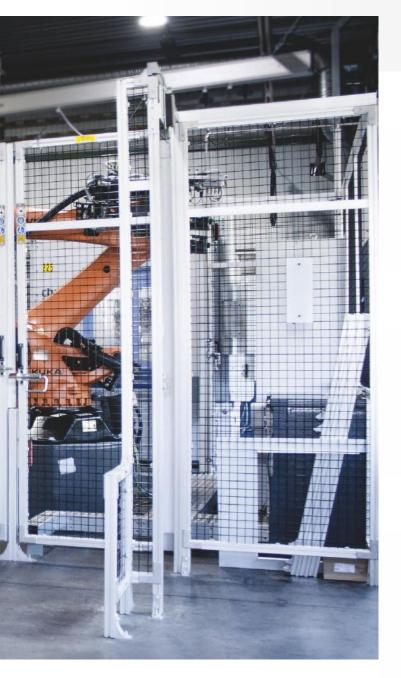
The combination of floor attachment bracket and aluminum profile easily compensates for any unevenness.
